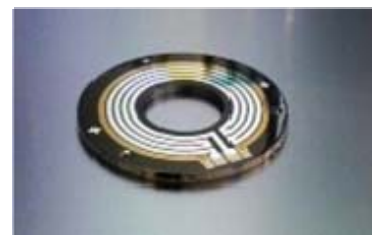
Fig. 3 Photograph of Pressure- and Temperature-Measuring Elements
