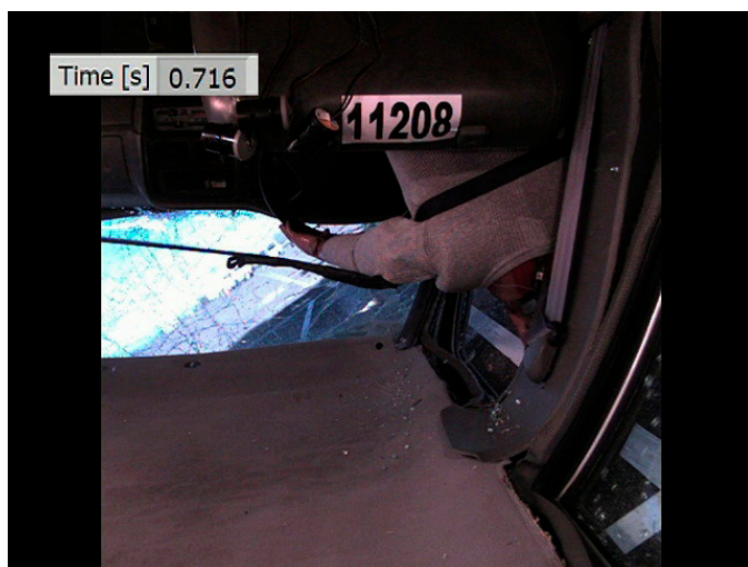
Figure 10: Onboard video showing the head-to-ground contact during the second impact in the Rodeo CRIS test.
