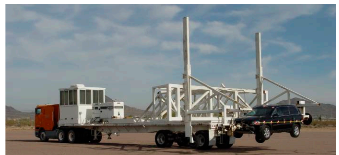
Figure 9: Photograph of CRIS system with vehicle attached.
