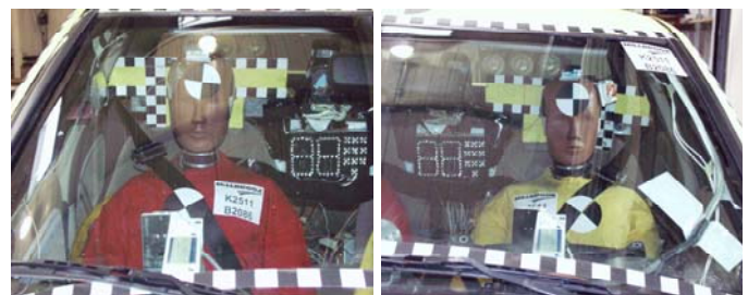
Figure 3: Position of the driver and passenger Hybrid III dummies and interior instruments and targeting.
