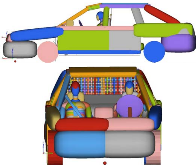
Figure 4: Madymo vehicle and occupant model of the friction rollover.
