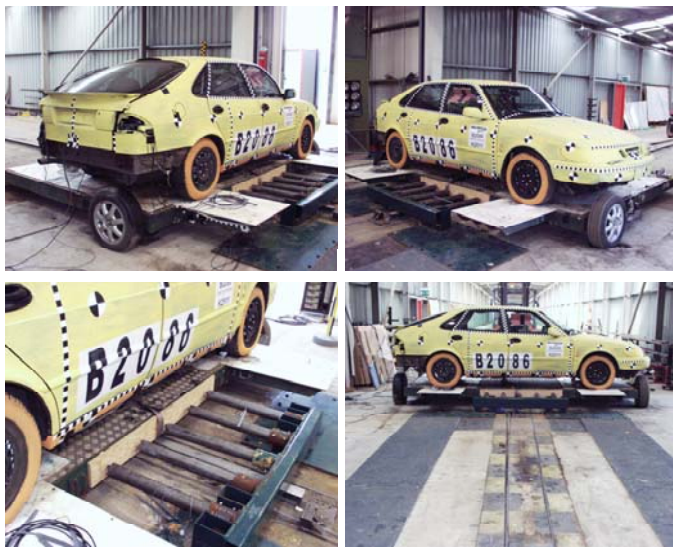
Figure 1: Test setup with the vehicle on a dolly that allows the vehicle to drop onto a high friction surface (MBK #B2086, Saab #K2511, June 5, 2000).
