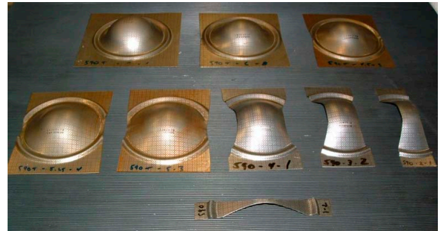
Figure 1: Samples formed using the traditional NA technique for determination of FLC ISO 12004-2 TECHNIQUE
