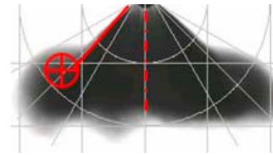
Figure 4: Spray Formation Recirculation Zone
