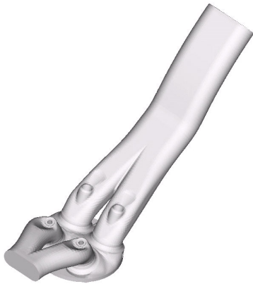
Figure 3. The simulation domain of a D35 EcoBoost engine
