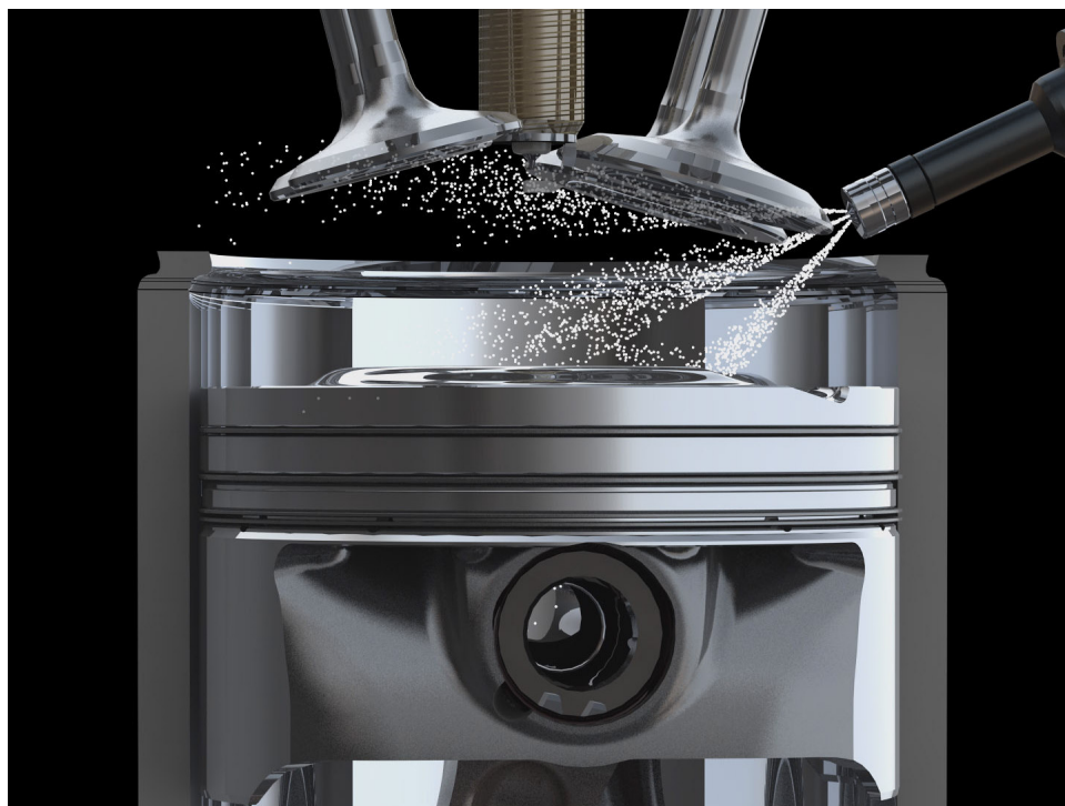
Figure 1 Schematic of the 3.5L V6 EcoBoost Combustion System.
