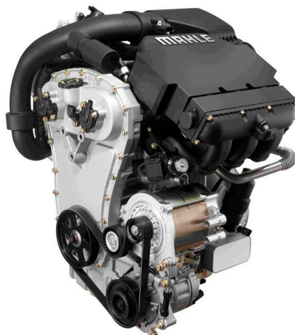
Figure 1: The downsized concept engine showing highly integrated design of intercooler, oil cooler/filter module and engine-mounted air cleaner.
