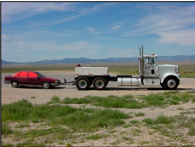
Figure 2. Rollover test configuration of tow vehicle (MMB) and vehicle used for tests #4 and #5.
