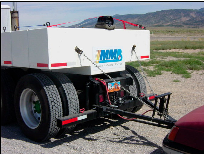
Figure 3. Release tow hitch mechanism attached to rear of tow vehicle (MMB).
