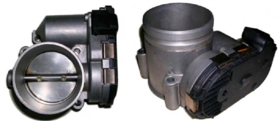
Figure 1: Picture of Bosch motorized throttle body (DV-E5)
