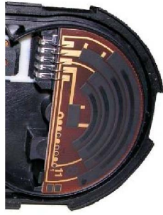
Figure 3: Embedded resistive throttle plate position sensors
