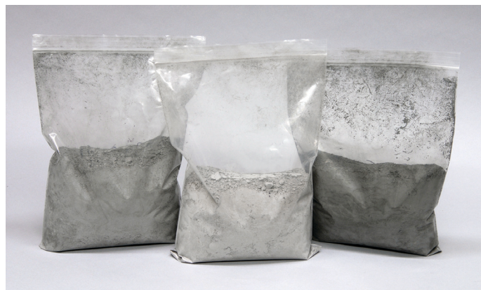
Figure 9. Typical bags of incombustibles received from test site after each DPF cleaning.
