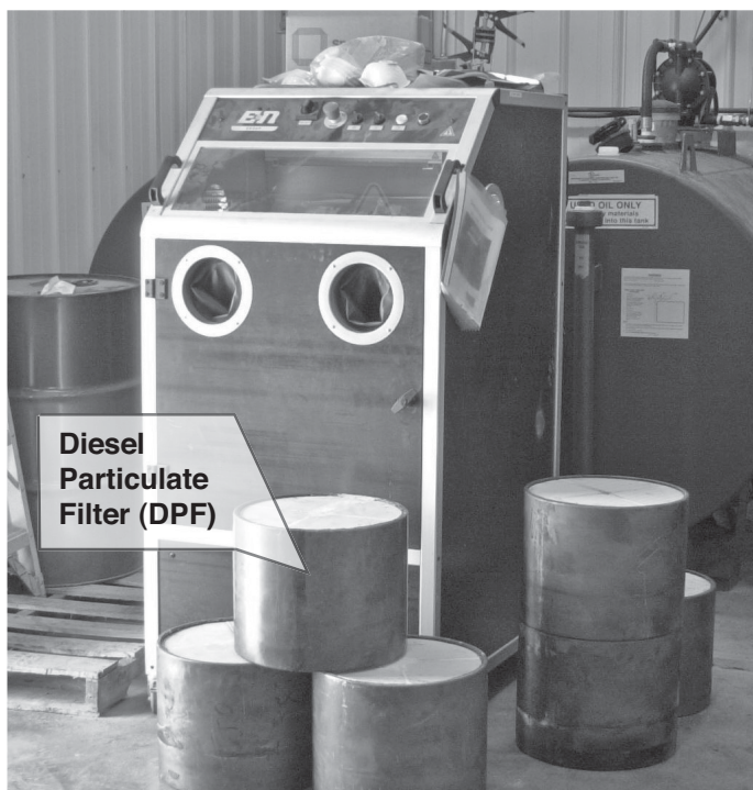
Figure 7. DPFs waiting to be cleaned in front of the cleaning equipment. The DPF size was 12 inches (30 cm) in diameter by 15 inches (38 cm) long.
