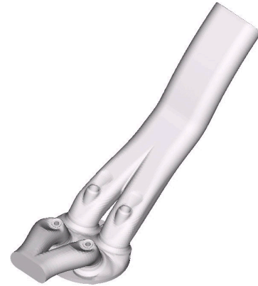
Figure 6. The simulation domain of a D35 EcoBoost engine
