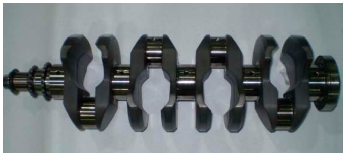
Figure 1: Crankshaft with 8 counterweights
