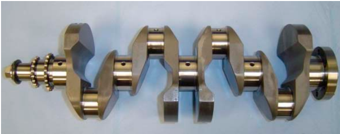
Figure 2: Crankshaft with 4 counterweights
