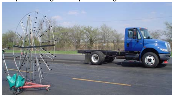
Figure 1: Ninety element acoustic beamforming array installed at the ITE test track
