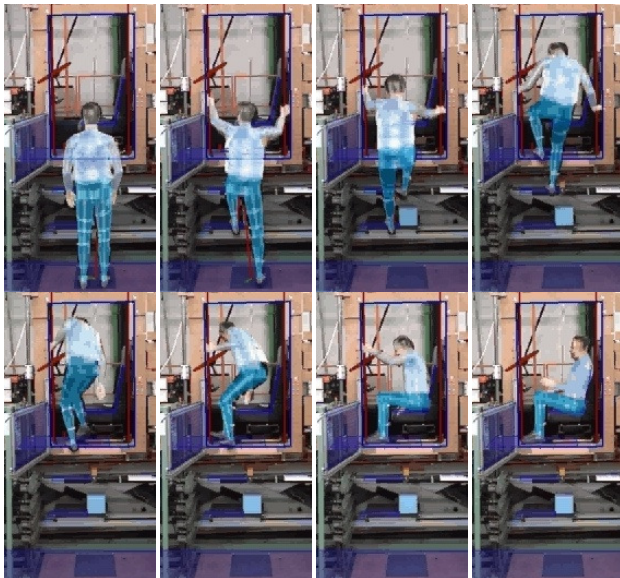
Figure 2. Reconstructed ingress motion super-imposed on a video of the motion.
