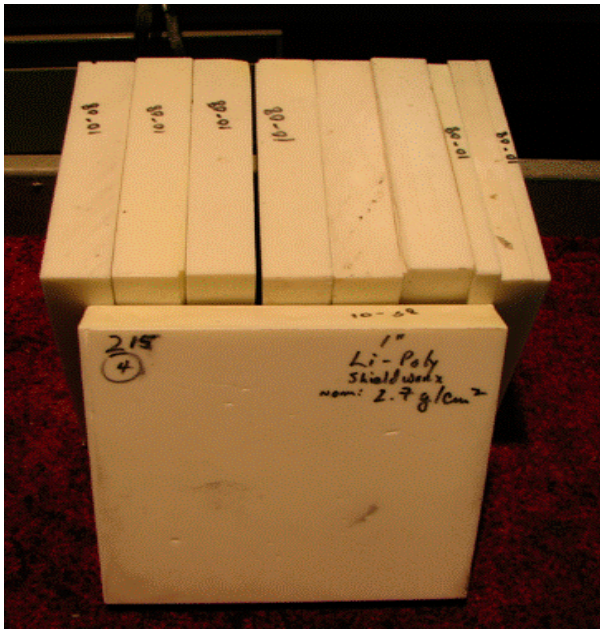
Figure 2: Sample coupons of lithium doped polyethylene (92.5% polyethylene, 7.5% lithium). The samples had dimensions of 15.24 cm x 15.24 cm (6" x 6") and the blocks were of various thicknesses. There are a total of ten coupons for this type of material. Combinations of the various thicknesses of this and the other samples described in Figs. 3 and 4 were used to achieve the desired density thickness for a particular shielding experimental run.
