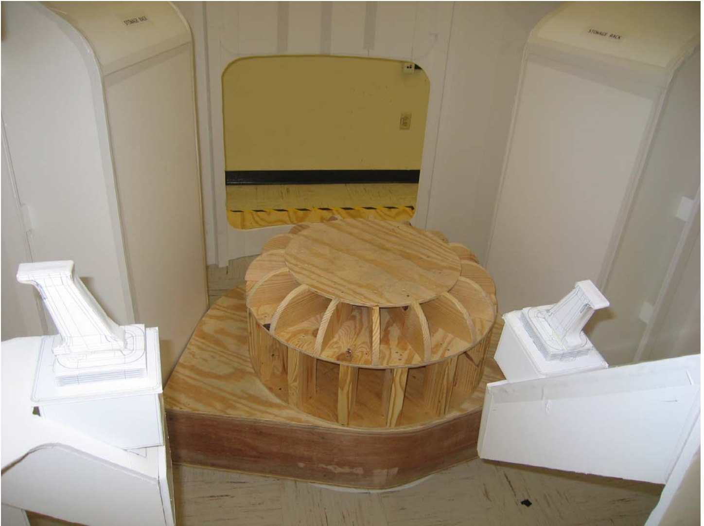
FIGURE 5. Detail of the Interior of the Ascent Module, 2006, showing the EVA hatch in approximately the same position as on the Apollo LM, behind the top of the ascent engine head shell. Photo credit: author, December 2006.
