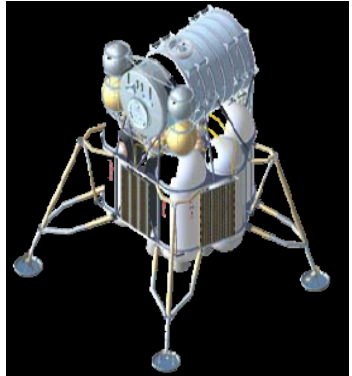
FIGURE 3. NASA Lunar Architecture Team LAT-1 concept for LSAM Concept A with combined Airlock and Habitat; it has a separate Ascent Module. Credit: NASA.
