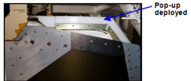
Figure 4. Side view of CQ top showing the pop-up deployed configuration.
