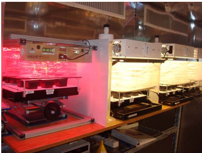
Figure 1. VEGGIE chamber with LED lighting (left) and BPSe chambers with compact fluorescent lamps (center and right) were used to determine feasibility of sustaining salad crop production through multiple growth cycles.
