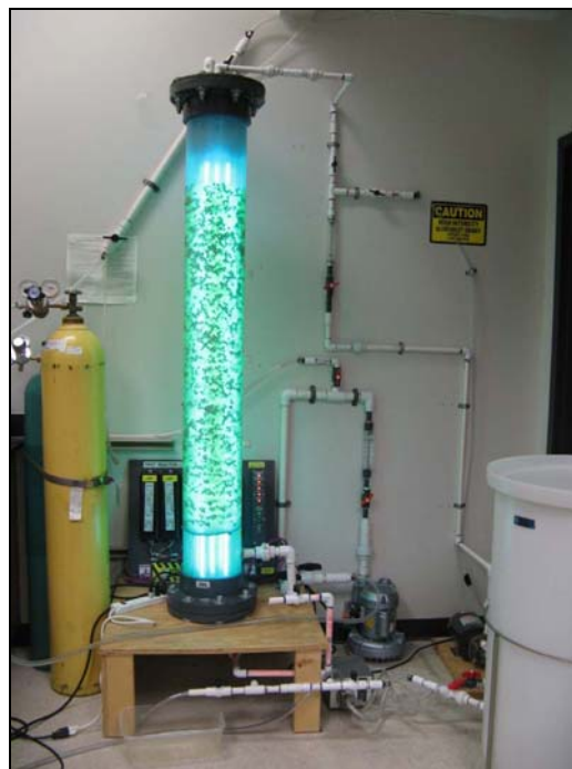
Figure 3. Picture of the two – phase photocatalytic reactor and experimental setup.
