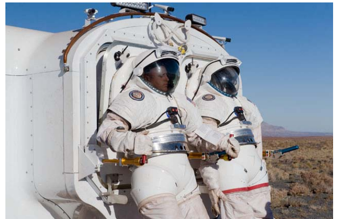
Figure 3 (jsc2008e139052): Suit Port Concept Evaluator on LER with Mark III Mockup Suits and the Port Side Test Subject Disconnecting from the Suit Port
