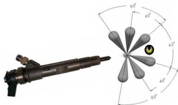
Figure 2: Spray geometry of the common rail injector CRI1
