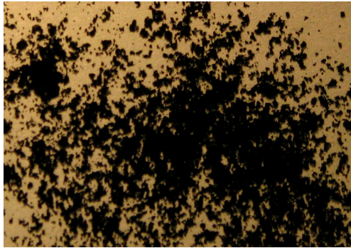
Fig.3 Soot particles collected from surface layer of deposit.
