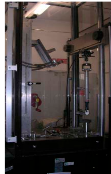
Figure 3: MTS Shock Absorber Test System adopted by PAIOLI MECCANICA to obtain the fork dynamic characteristics.
