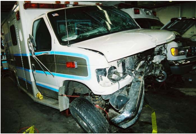
Figure 3. Frontal impact damage to the ambulance
