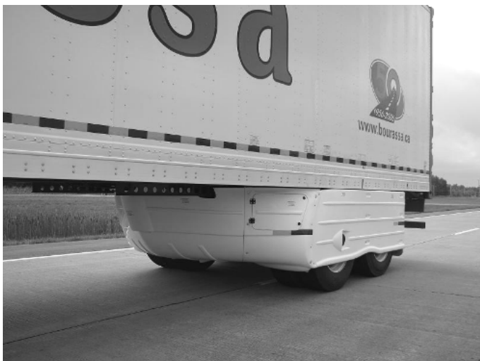
Figure 2. Trailer axles' deflector
