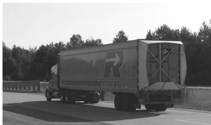
Figure 3. Trailer rear deflector
