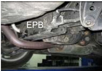
Fig. 4 Installation examples of cable puller EPBs.
