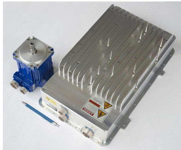
Figure 4: Electric Motor and Power Control Electronics
