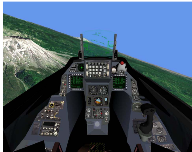
Figure 1. A virtual cockpit for the F-16, made with DiSTI's GL Studio tool. The instruments in the cockpit are composed of 2-D geometry, overlaid with photorealistic textures. The textures were created using source images of the actual instruments.
