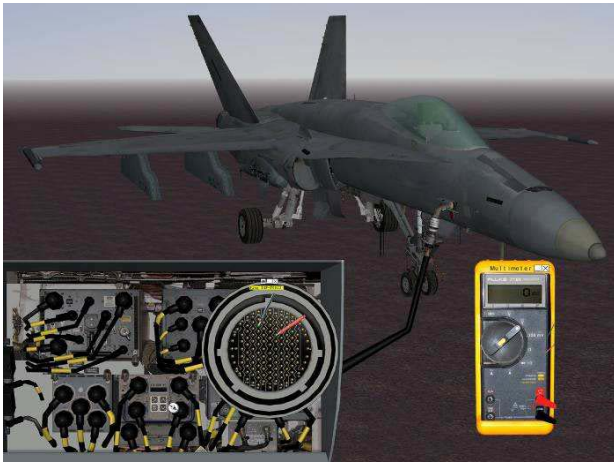
Figure 2. A Virtual Maintenance Trainer for the FA-18. The models of the jet and the support equipment were developed with extensive source images from the actual aircraft.
