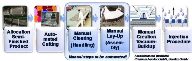
Figure 2: Basic process chain in the manufacturing of dry carbon fibre textiles
