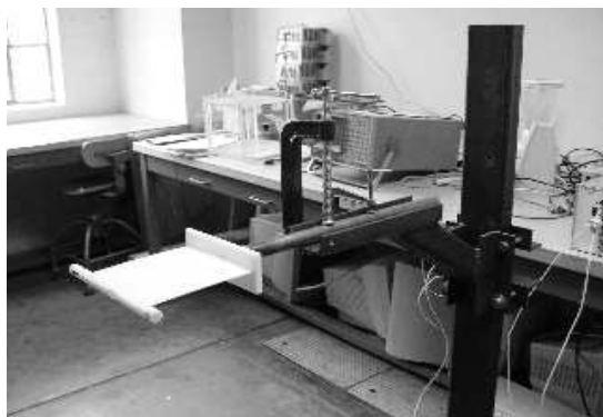
Figure 2. Airfoil model manufactured using rapid prototyping
