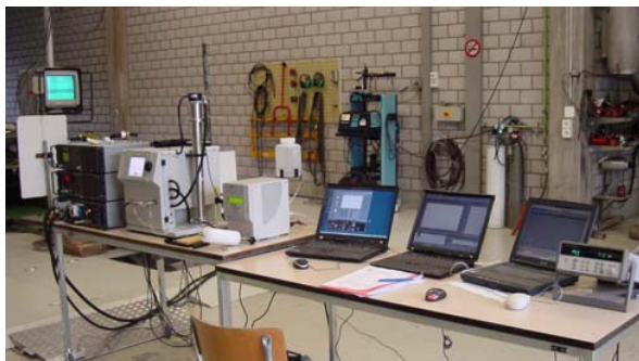
Fig. 2: Sampling and measuring set-up for nanoparticulate analysis of scooters.
