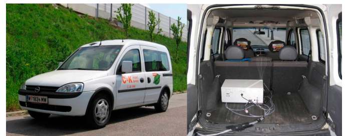
Figure 5: Light duty test vehicle with the OBM device
