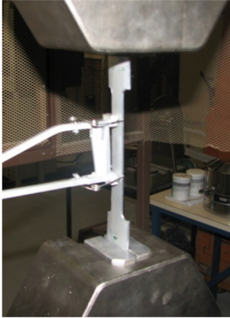
Figure 2. Tensile testing of a dog-bone specimen cut from a tube.
