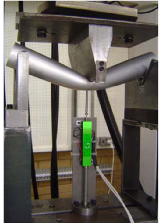
Figure 1. A foam-filled tube under three-point bending.
