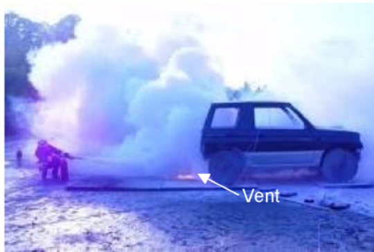
(b). Test 7, 45 deg. diagonal backward vent, Dry powder extinguisher
