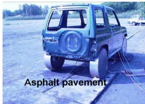
Figure 2. Vehicle simulator and asphalt pavement
