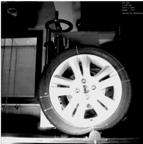
Figure 3. Principal setup and operation of Fraunhofer LBF large deformation test rig
