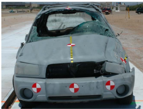
Figure 19. Roof deformation to Subaru Forester after the test on concrete.
