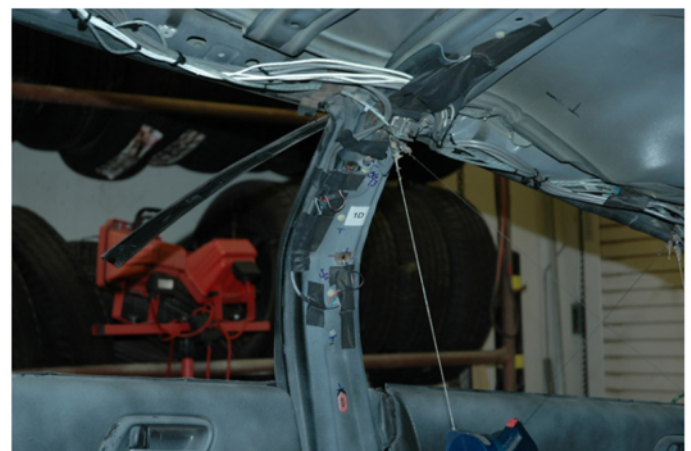
Figure 13. Interior of left B-pillar post-test on dirt without ATDs.
