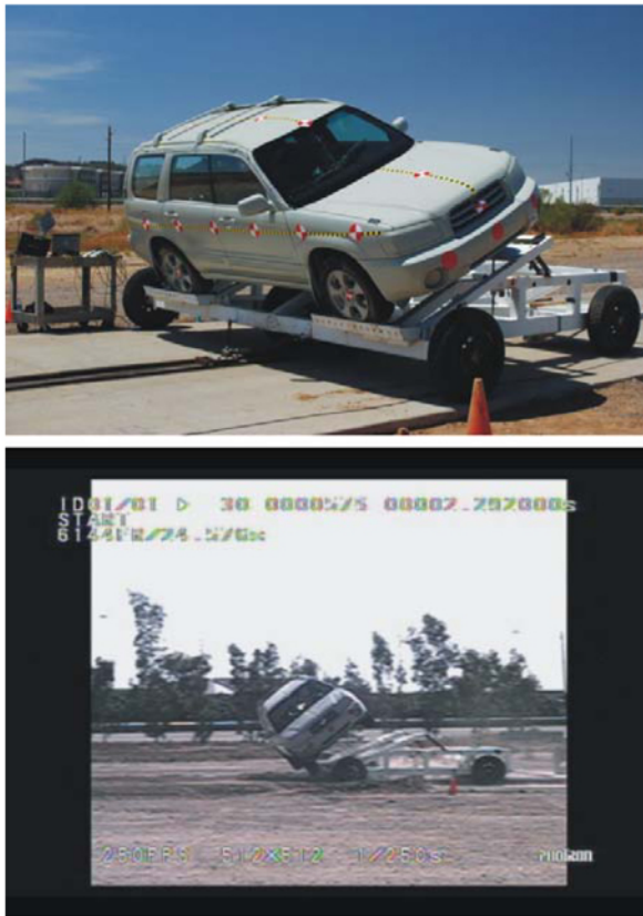
Figure 6. Still photographs of test vehicle on rollover dolly (top), and frame capture from high-speed video depicting vehicle at separation from rollover dolly (bottom).
