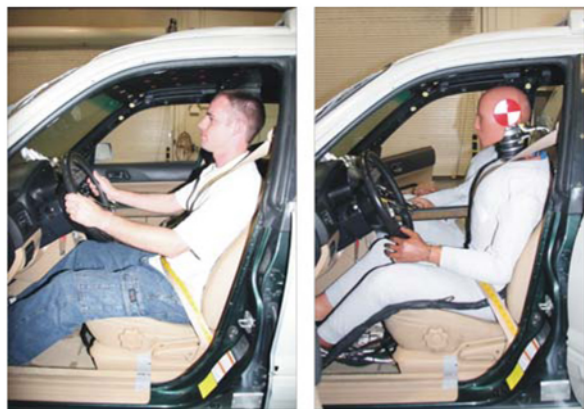
Figure 1. Head clearance and belt length measurements were recorded with the vehicle in the upright position for both the human surrogate (left) and ATD (right).
