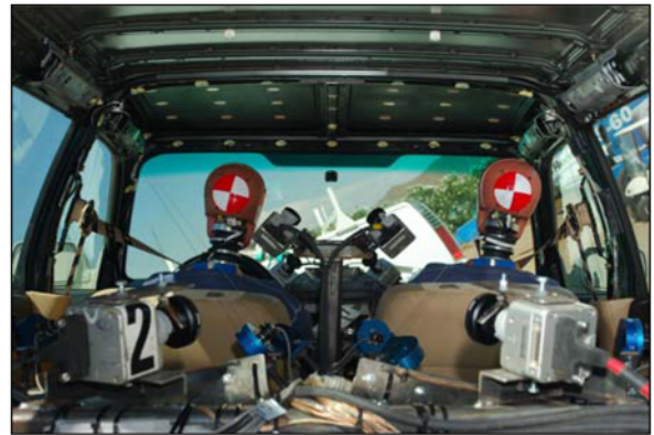
Figure 4. Depiction of ATD and onboard camera positions.
