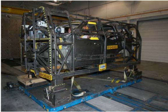
Figure 7. Rollover Component Test System (ROC)
