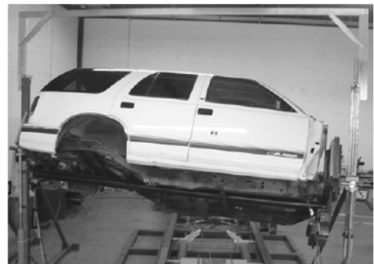
Figure 4. Jordan Rollover System with Vehicle Mounted and Ready for Testing
