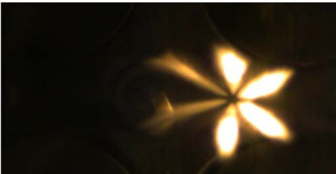
Figure 6. Image taken using the halogen lamp, inlet valves located at the bottom of the image
