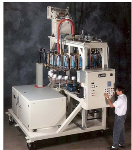
Figure 4. Carousel induction heater for billet re-heating
