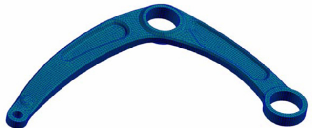
Figure 3. Finite element model of the lower control arm
