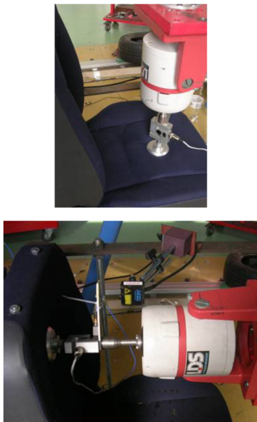
Fig. 6. Seat damping measurement.
