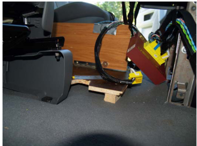
Figure 3. ACM module and top panel rotated approximately 90 degrees, causing a deployment event.
