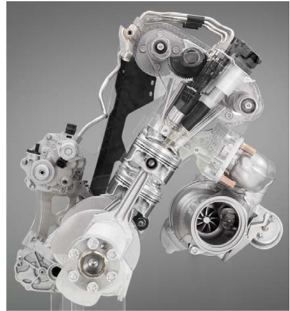
Fig. 2. The new BMW six-cylinder engine concept with turbocharging and the Valvetronic CVVL system [8]
