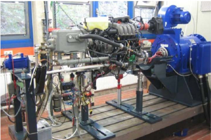
Fig. 4. Test rig application with the 2.0l Audi engine and UniValve
