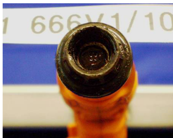
Figure 16. Injector deposits after 60 hours with unadditized E85 / with EGR and blow-by
