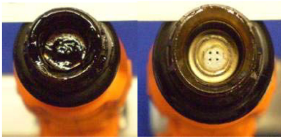
Figure 10. Visual rating of injectors. Dirty Injector (left) and Clean Injector (right)
