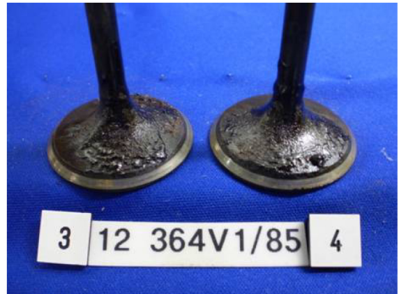
Figure 11. IVD after 60 hours with unadditized E85
