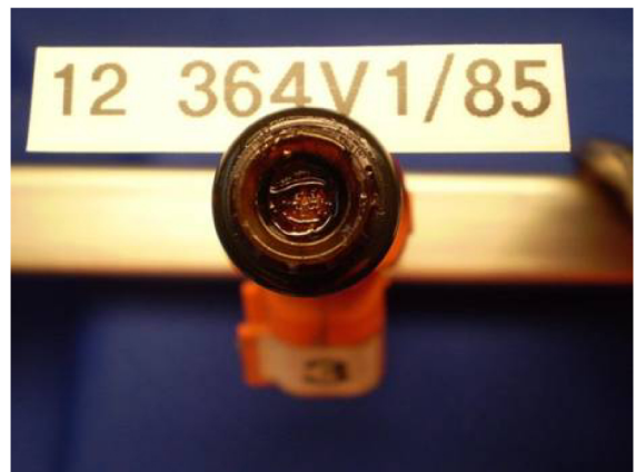
Figure 12. Injector deposits after 60 hours with unadditized E85
