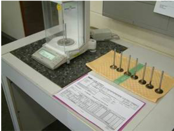
Figure 9. Deposit mass determination of IVD
