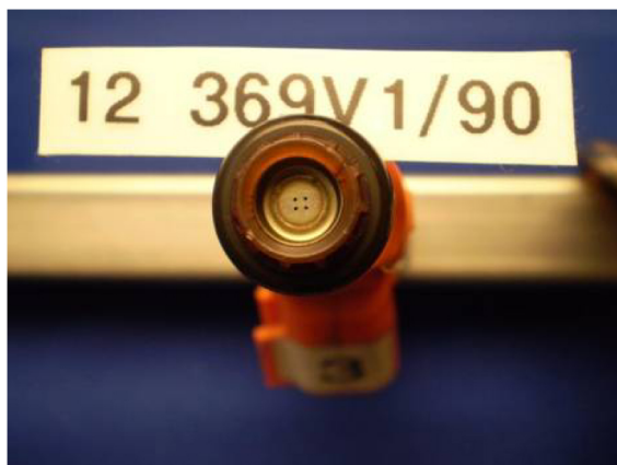
Figure 14. Injector appearance after 60 hours with unadditized E0
