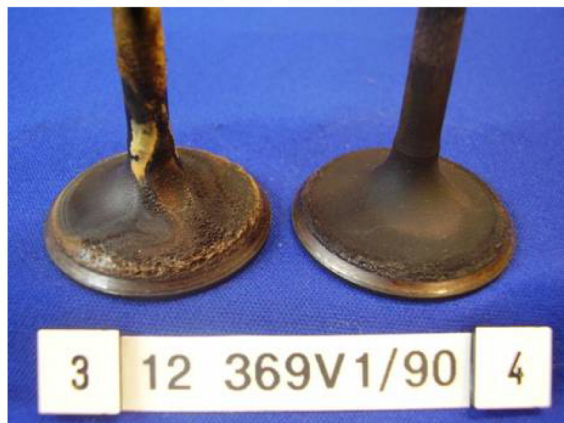
Figure 13. IVD after 60 hours with unadditized E0
