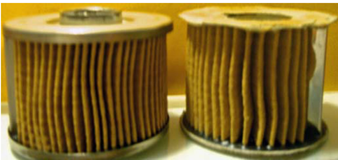
Figure 5. Comparison of Cardboard and Steel End Caps.
