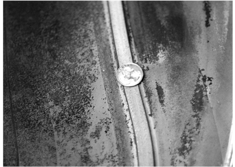
Figure 1. Typical SPF die surface after numerous thermal cycles at 900°C.
