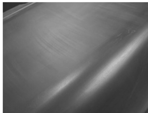
Figure 6. Surface of SPF die for forming fine grain 6A1-4V after several years of production and numerous thermal cycles [1].
