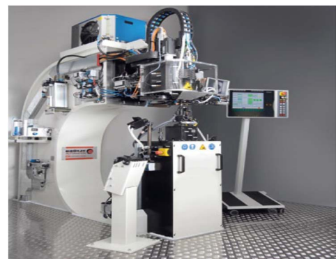
Figure 6. The riveting machine
