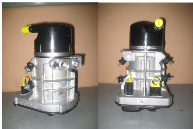
Figure 4. 100CV EPHS Unit
